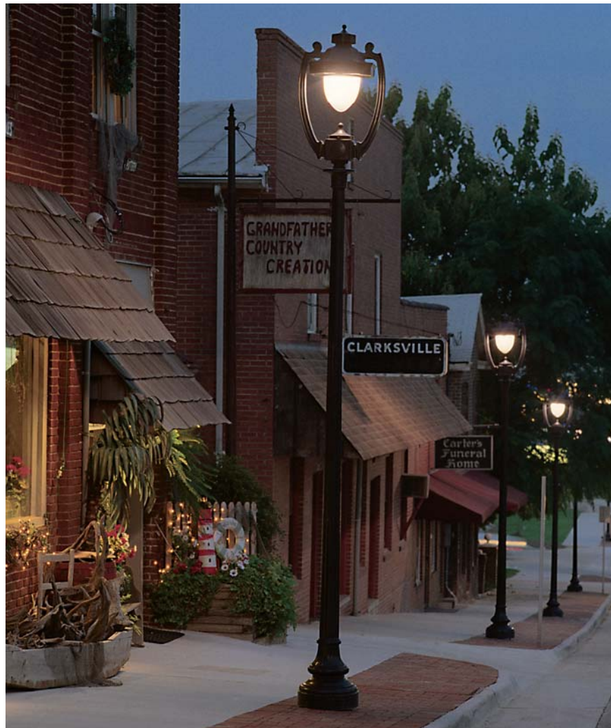
Figure 1 The non-optical globe produces maximum light output at 90° thus creating disabling glare and wasting the majority of available light.
