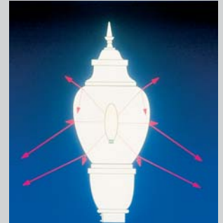
Figure 2 The prismatic acorn redirects light to maximize efficiency and limit glare.
