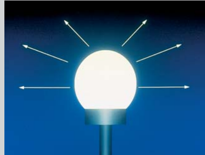
Figure 1 The non-optical globe produces maximum light output at 90° thus creating disabling glare and wasting the majority of available light.
